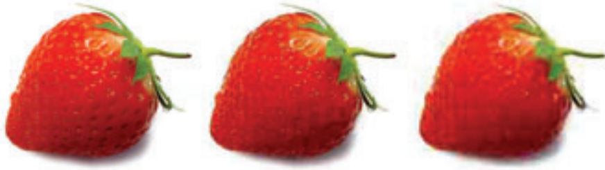
Figure 5.20: An image of a strawberry saved at increasing levels of JPEG compression
